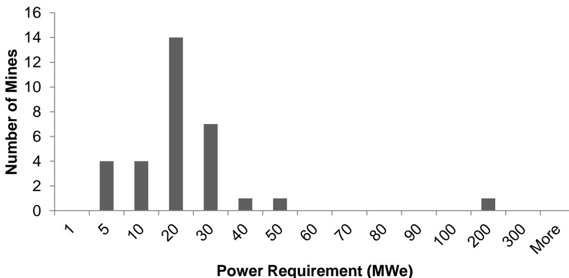
Figure 4. A histogram of power requirements of off-grid mines in Canada
