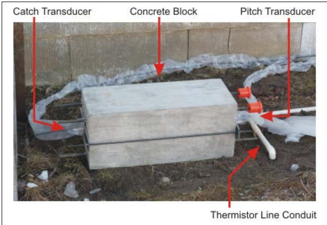
**Figure 1: Initial Ultrasonic Pulse Velocity Experiment**
