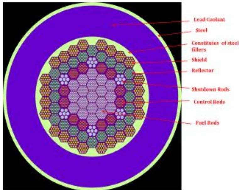
**Figure 1: The SEALER Core Layout in the SERPENT Model**
