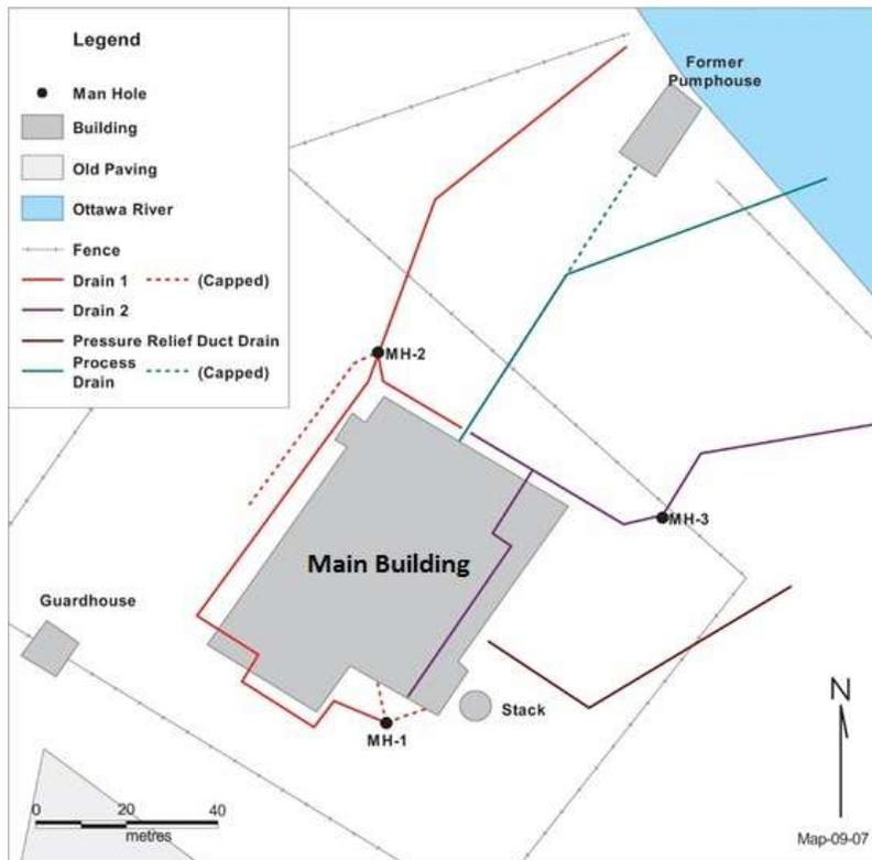
Figure 3: Active and inactive drainage systems around the NPDWF
